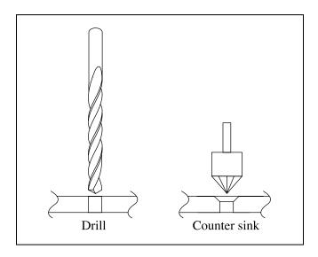
Figure 13. Drill and counter sink insert.
